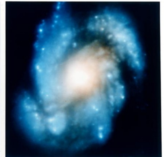
Image with Spherical Aberration
