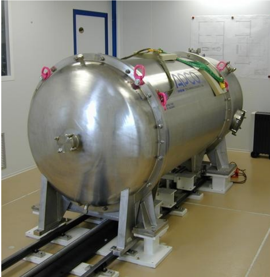
Komora próżniowa spektrografu HARPS (High Accuracy Radial velocity Planet Searcher).
